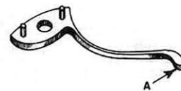
Brake Lever Spring Assembly No. 20
